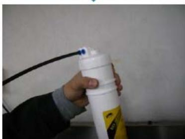
6. Connect the other side of tube into inlet of new filter
