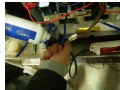
3. Connect it into outlet of sediment filter
