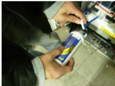
2. Disconnect the tube from filter
