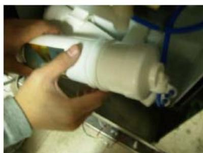
2. Disconnect the tube from filter
