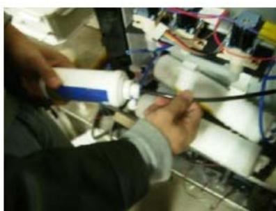
4. Connect it into outlet of sediment filter
