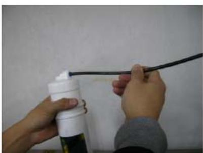
5. Connect the other side of tube into outlet of new filter
