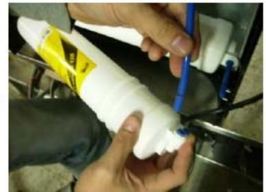
3. Disconnect the tube & flow restrictor for brine water
