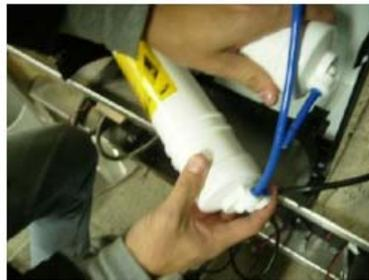
2. Disconnect the tube from filter
